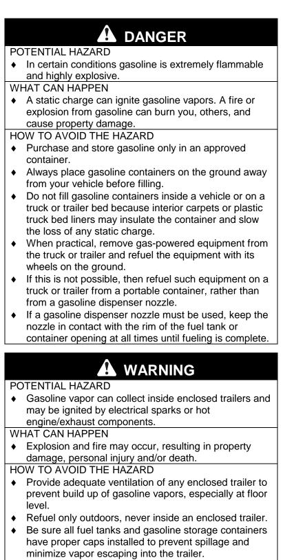
Do not place any equipment that is leaking gasoline in an enclosed trailer.
